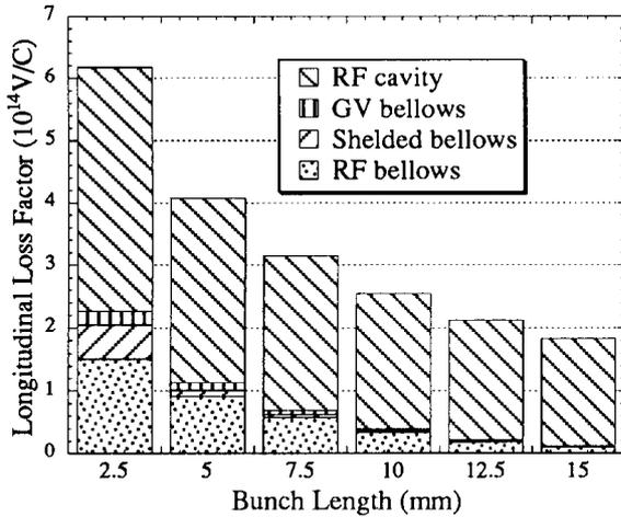
Fig. 2 Longitudinal Loss Factor Computed with ABCI
