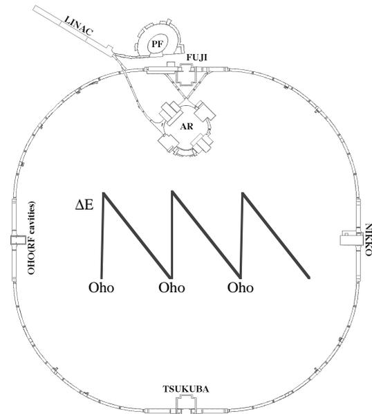
Fig. 1 Layout and Energy Saw of TRISTAN MR
