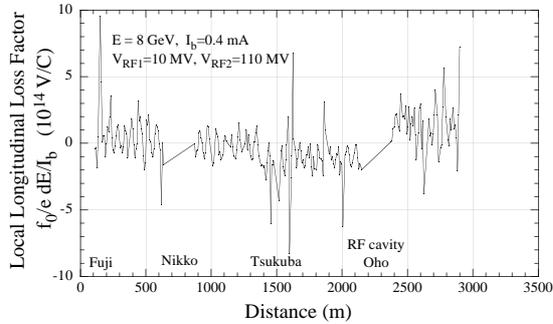
Fig. 5 Measured Differential Longitudinal Loss Factor
