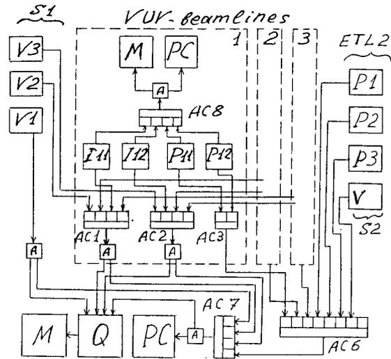
Fig. 2. Beam diagnostics in booster S1, VUV beamlines, and ETL2 line: V1-V3 visual-light TV cameras of the S1 booster; A- matching amplifiers; I11, I12- imaging ionization detectors of the first VUV beamline; P11, P12-phosphor probes of the same beamline; M- television monitor; PC personal computer; Q- quadrator; AC1-AC3, AC6-AC8 analogue commutators; P1-P3 phosphor probes of the ETL2 line; V visual-light TV pickup camera on the S2 ring.
