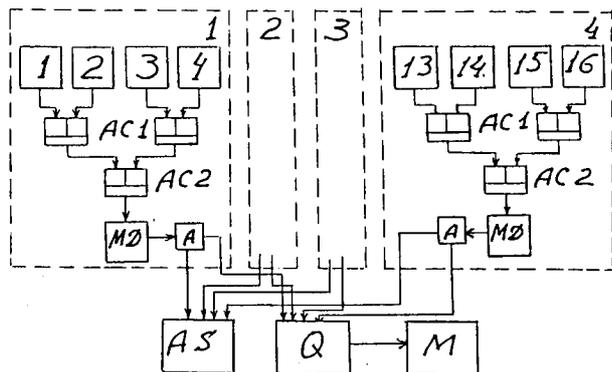
Fig. 4. Block diagram of a branch of TV room-survey system (16 channels): 1-16 visual-light survey TV cameras; AC1, AC2- analogue commutators; A- matching amplifier; AS- alarm signal switch; Q- quadrator; M- monitor.
