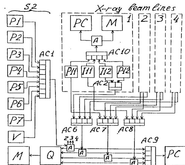
Fig. 3. Block diagram of a beam-diagnostics branch (S2 storage ring and four x-ray beamlines):P1-P7 Phosphor probes of the S2 ring; V visual-light TV pickup camera of the S2 ring; P11, P12 phosphor probes of an x-ray beamline; I11, I12 imaging ionization detectors of the same beamline; AC-analogue commutator; A- matching amplifier; M- monitor; Q- quadrator; PC personal computer.
