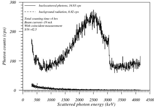
**FIG. 3**  $\gamma$ -ray spectrum of Compton scattering with collimator of 3mm diameter under synchronous measurement. (electron beam current=19mA, counting time=4hrs., and  $S/N$  ratio =42.5.)
