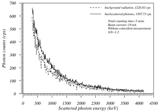
**FIG. 5**  $\gamma$ -ray spectrum of Compton scattering with collimator of 3mm diameter and without synchronous measurement. (electron beam current=19mA, counting time=5mins., and  $S/N$  ratio =1.2.)
