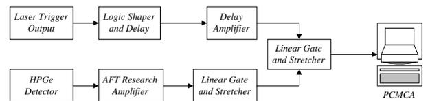
**FIG. 2** Instruments associated with synchronous measurement.
