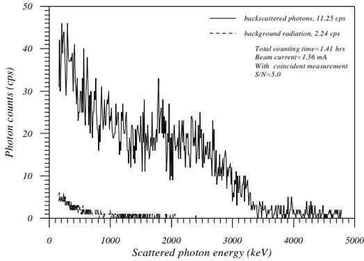
**FIG. 4**  $\gamma$ -ray spectrum of Compton scattering with collimator of 10mm diameter under synchronous measurement. (electron beam current=1.56mA, counting time=1.41hrs., and  $S/N$  ratio =5.0.)
