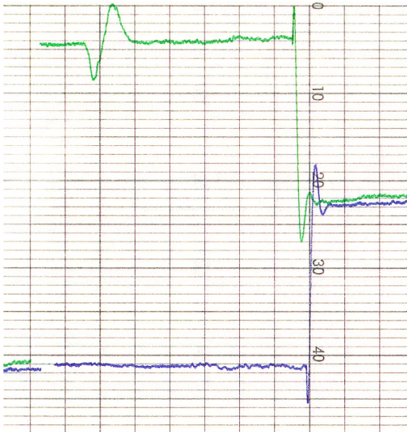
Fig. 6. Calibration of scale. The connection between the vessels is closed and 1\text{cm}^3 of water is added to one vessel. Then the connection is opened and the levels equalised. 1\text{cm}^3 equals 0.1\text{mm} .
