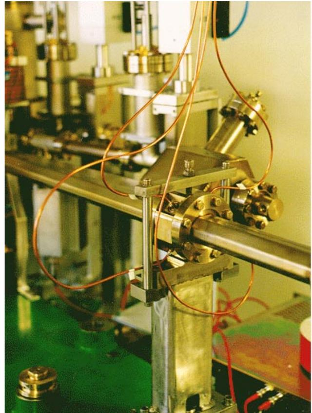
Fig. 1. A BPM head in MAX-II mounted on its rigid support pillar on a girder before mounting of the magnets.
