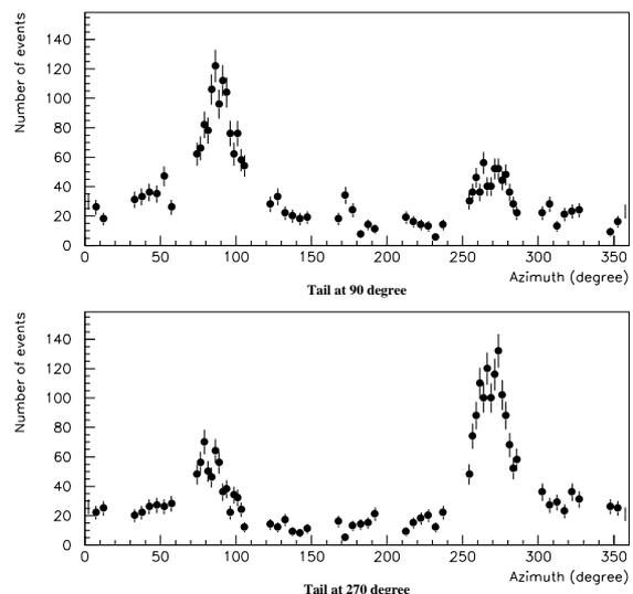
Figure 4: Azimuthal distribution of  $\text{He}^+$  ions with a horizontal tail at  $90^\circ$  (top) and  $270^\circ$  (bottom)
