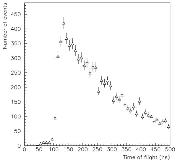
Figure 2: Time of flight spectrum of  $\text{He}^+$  ions (statistics for 400 electron bursts)
