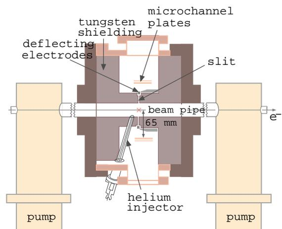
Figure 1: Longitudinal view of the monitor
