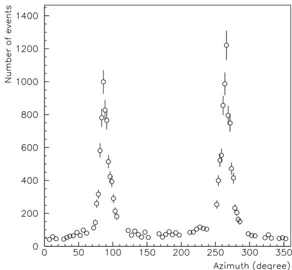
Figure 3: Azimuthal distribution of  $\text{He}^+$  ions corrected for the pile up. The azimuth origin is the upward direction
