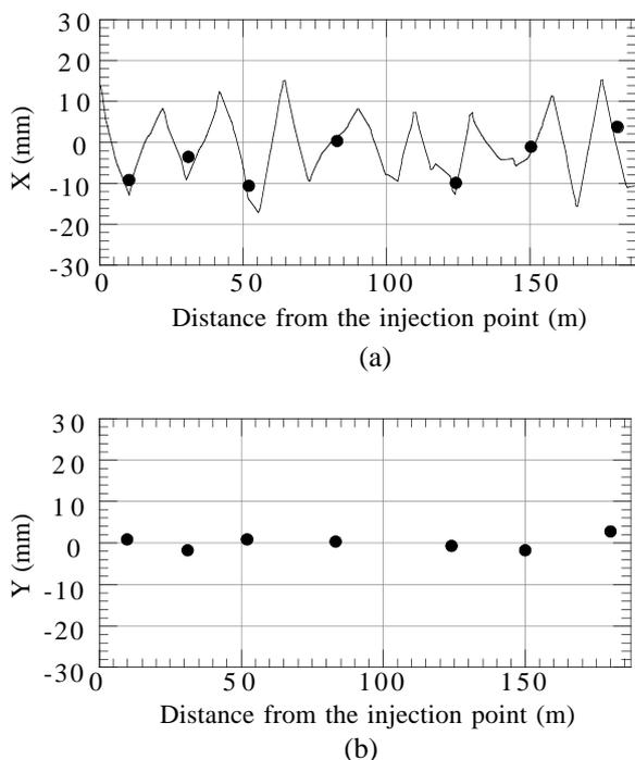
Figure 4 Injected-beam positions of the first turn. (a) horizontal beam positions. Solid line is the calculated orbit. (b) vertical beam positions.
