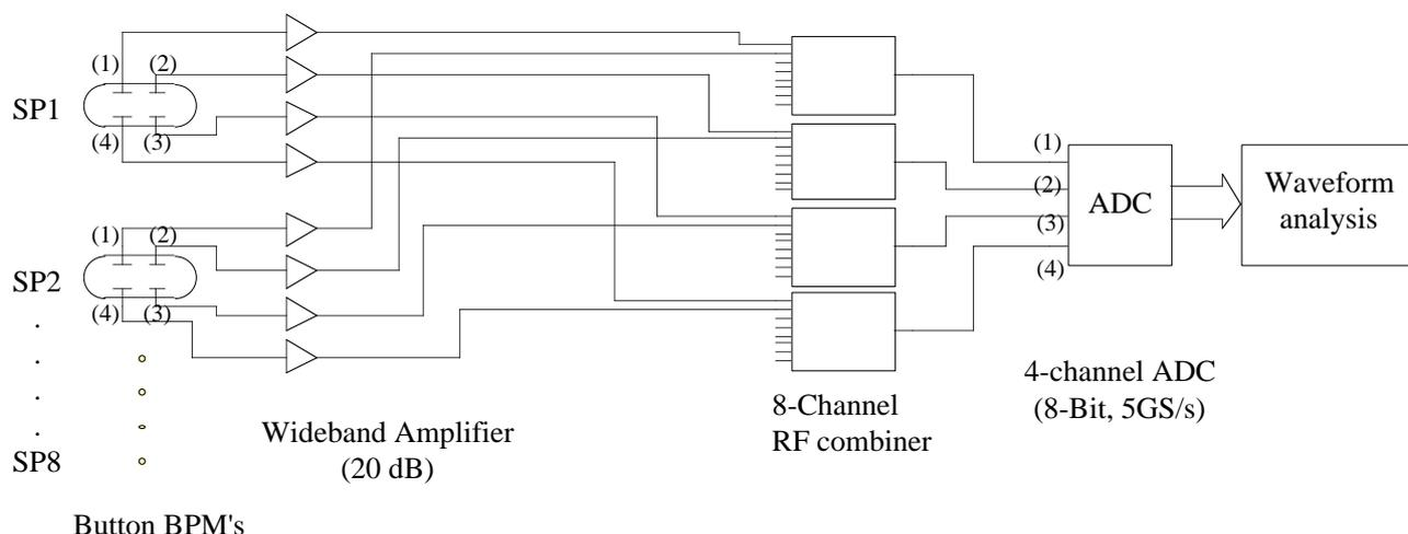
Figure 1 Signal processing scheme of the single-pass BPM system.
