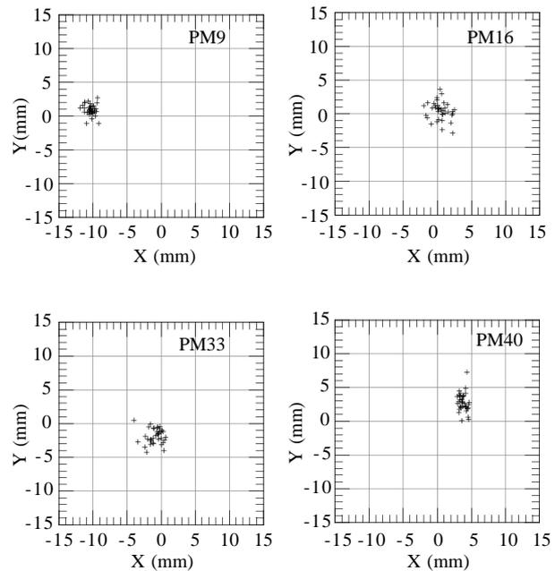
Figure 3 Examples of the beam-position measurements at the first turn in the ring. Distribution of the positions of 50 injection pulses were plotted in the each graph.
