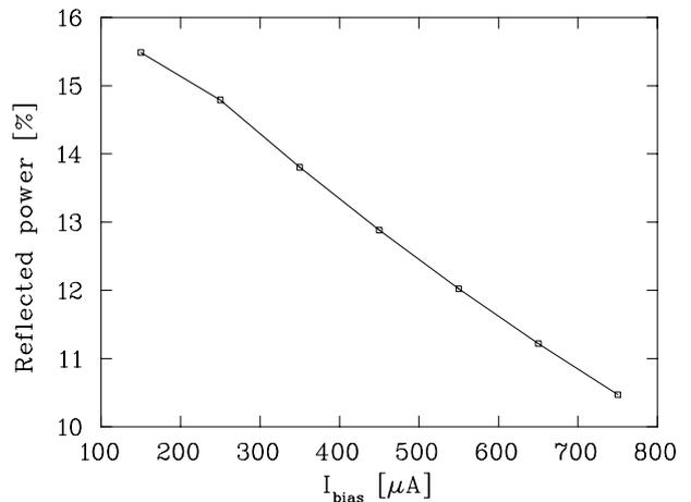
Figure 5: Reflected power as a function of the bias current.
