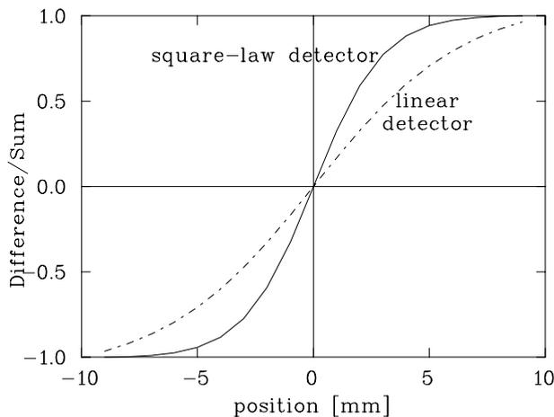
Figure 7: Calculated difference/sum as a function of position for a linear detector and for a square-law detector.
