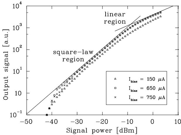
Figure 6: Measured output signal as a function of the input power for several different bias currents.
