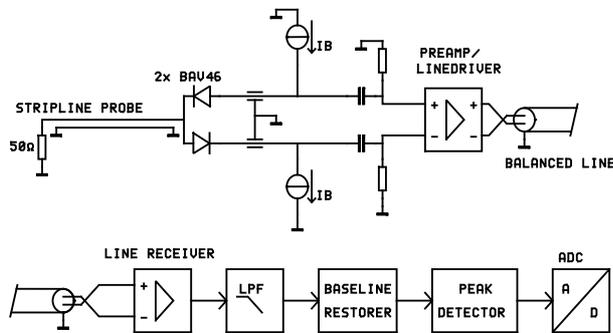
Figure 3: Block-scheme of the beam position monitor processing system.
