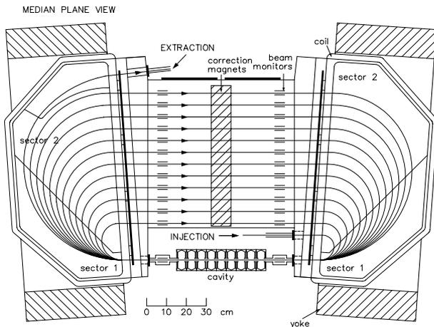
Figure 1: Racetrack microtron Eindhoven.
