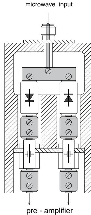
Figure 4: Copper-gilt housing of the microwave diode detectors. The signal conductors are marked gray.
