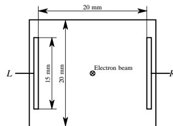
Figure 2: Cross-section of a stripline BPM.
