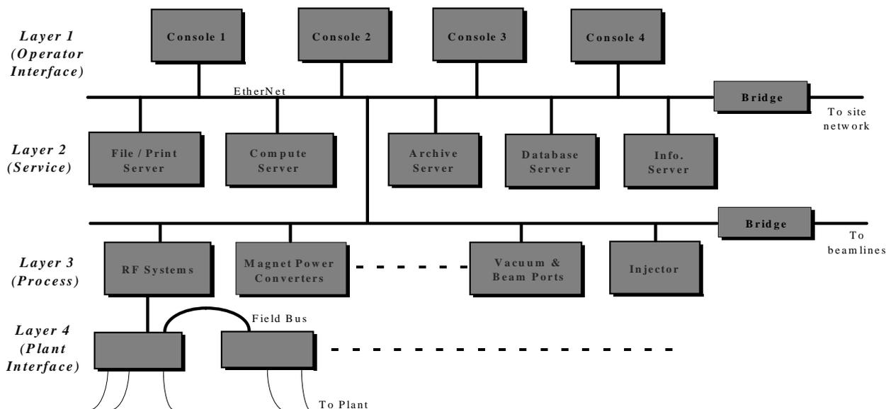
**Figure 1: Proposed Structure of DIAMOND Control System**
