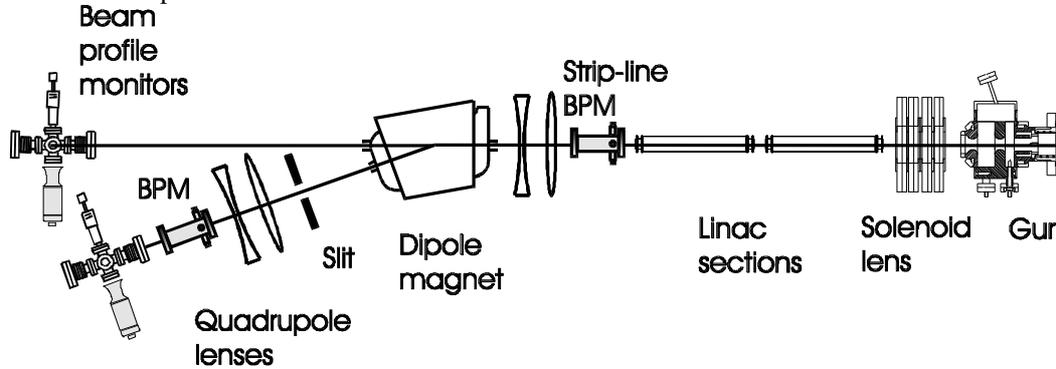
Figure 2. The schematic of ATF accelerator system.
