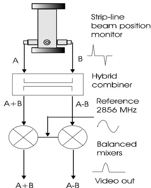
Figure 1. The stripline beam position monitor system.
