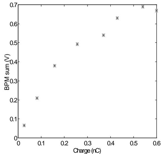
Figure 3. The BPM dynamics range characterization.
