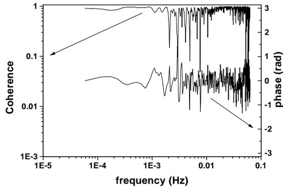
Figure 3: Coherence and phase difference between two sensors separated by 50 cm with an expansion joint.
