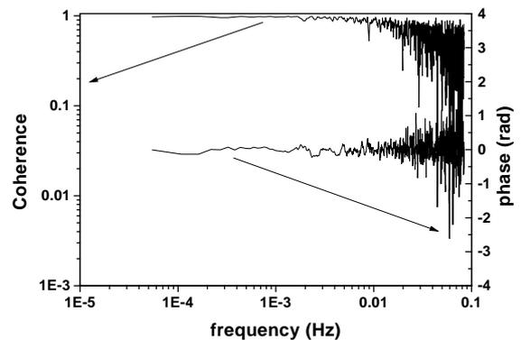
Figure 5: Coherence and phase difference obtained in the granite tunnel. Two levels were set up 46 meters apart.
