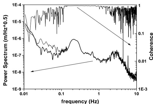
Figure 1: A typical example of the ground vibration in KEK. The spectra were observed by two seismometers at a distance of 48 meters.
