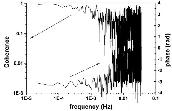
Figure 4: Coherence and phase difference obtained in the welded tuff tunnel. Two levels were set up 46 meters apart.
