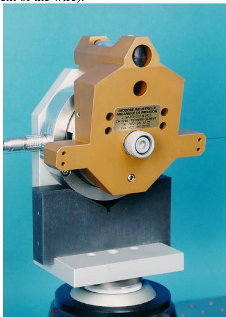
Figure 4: WPS captor adapted to standard reference with verticalizing tool.
