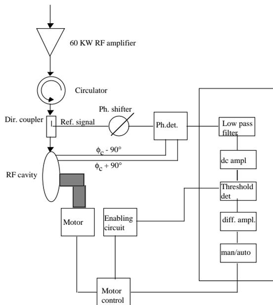
Fig. 1 Simplified block diagram of the tuning loop
