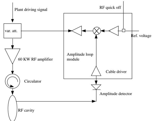
Fig. 2 Simplified block diagram of the amplitude loop
