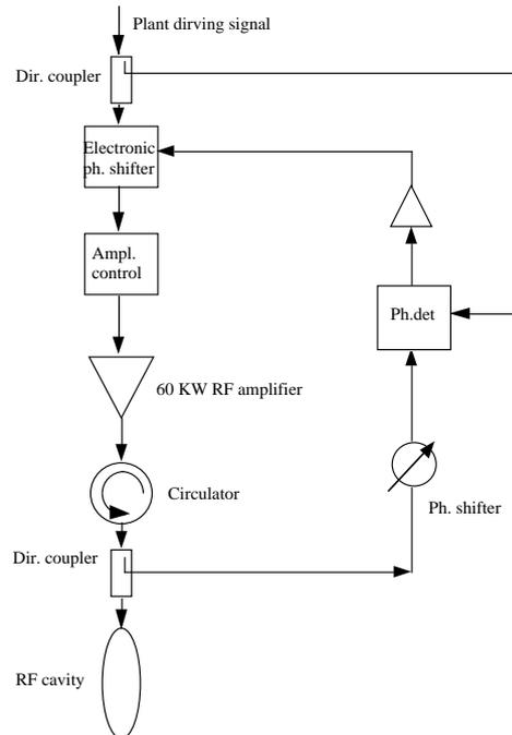
Fig. 3 Simplified block diagram of the phase loop
