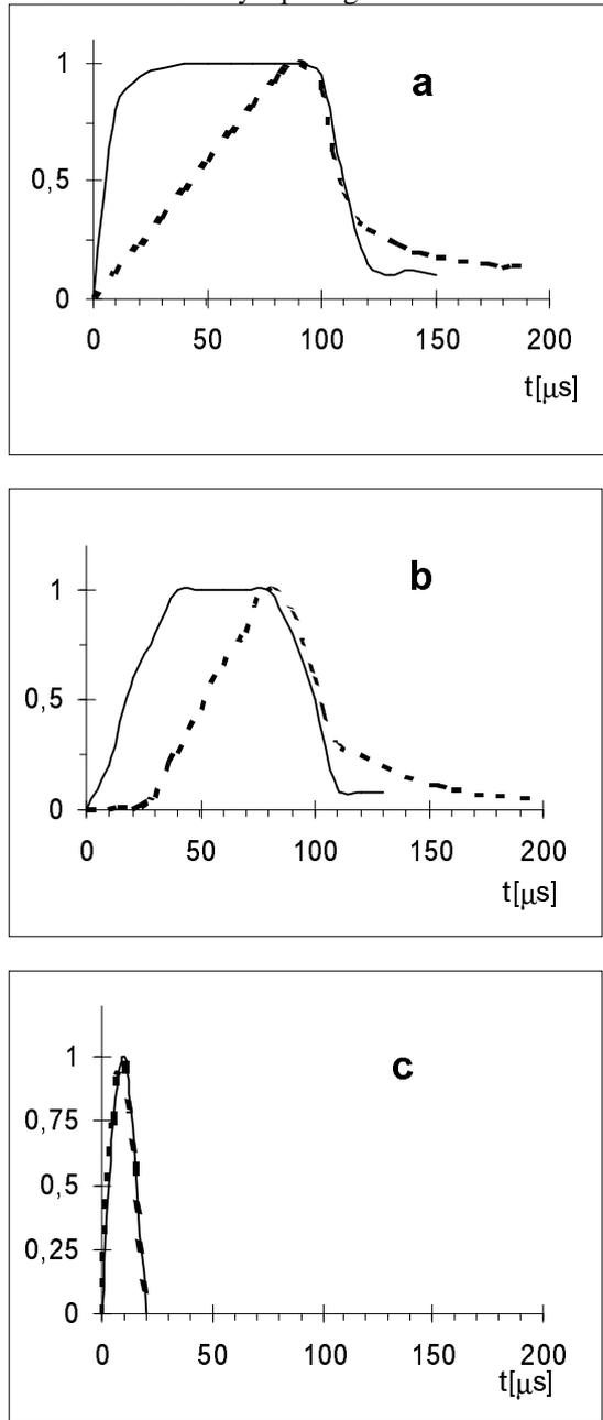
Fig. 1. The normalised current signal from photomultiplier (dashed line) and RF-power signal (solid line) time-dependencies for two types of cavities: space homogeneous (a) and space inhomogeneous (b) RFQ;
