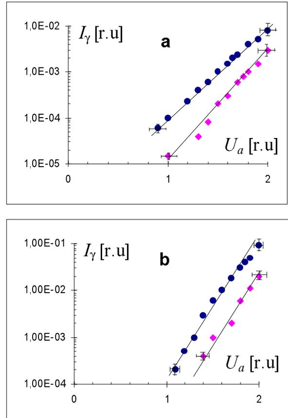
Fig.2. The light radiation intensity ( $I_\gamma$ ) vs RF power ( $U_a$  is the loop signal) for two types of cavities: space homogeneous (a) and space inhomogeneous (b) RFQ.
