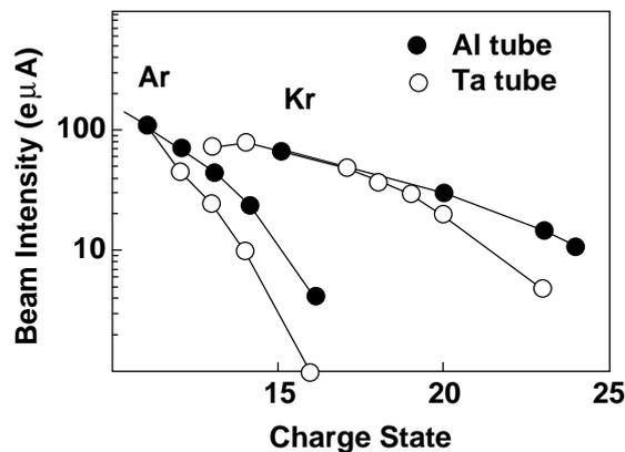
Fig.3. Charge state distribution of Ar and Kr ions. Open and closed circles represent the results obtained with a Ta and Al tube, respectively.
