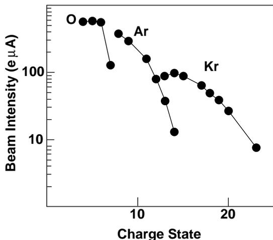
Fig.2. Charge state distributions of highly charged ions from gaseous elements.
