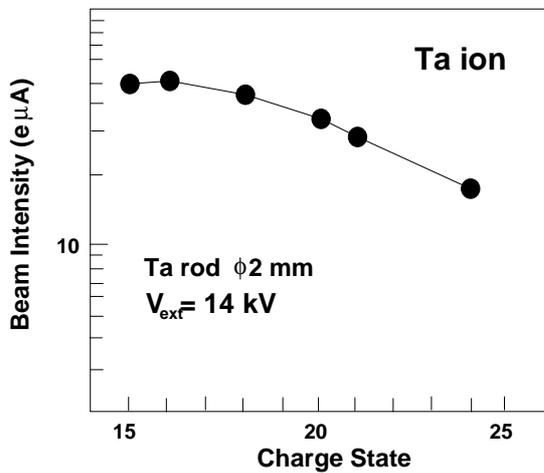
Fig.5 Charge state distribution of Ta ions at the extraction voltage of 14 kV
