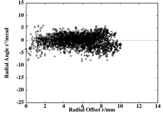
Figure 8: Transverse phase space of the first, middle and last bunch behind the solenoid (New design), gradients of the second and third cell increased to 120 MV/m.
