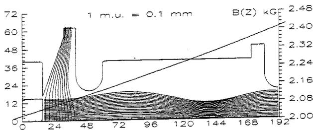
Figure 1. EGUN simulation of extraction of a 3 A electron beam from a 3 mm  $\varnothing$  CeIr cathode.
