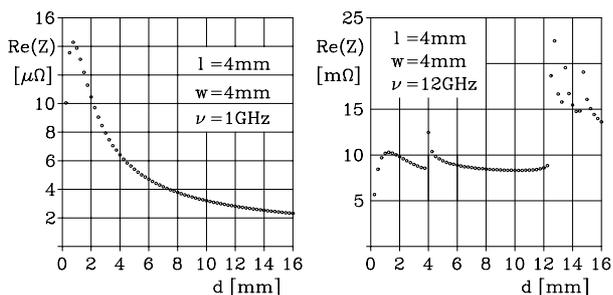
Figure 8: real part of impedance versus the distance  $d$  between inner and outer conductor at 1 GHz (left) and 12 GHz (right);  $b=16\text{mm}$
