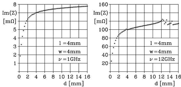
Figure 7: imaginary part of impedance versus the distance  $d$  between inner and outer conductor at 1 GHz (left) and 12 GHz (right);  $b=16\text{mm}$
