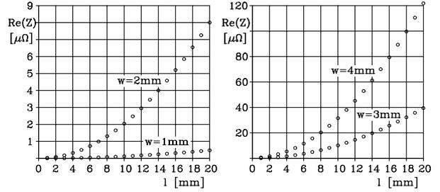
Figure 4: real part of impedance for slots with the width  $w$  and the length  $l$  at 1 GHz calculated by mode matching;  $b=16\text{mm}$ ,  $d=5\text{mm}$
