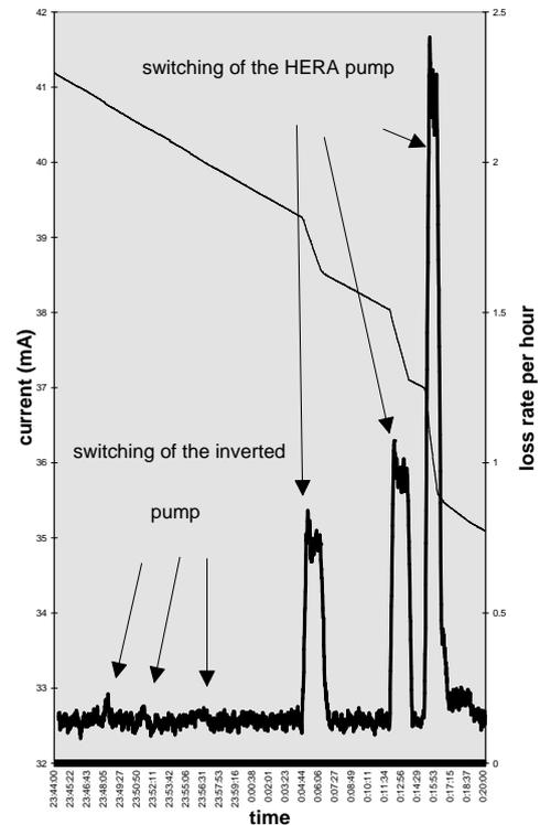
Fig. 4: Comparison of the effect of the inverted pump and the HERA pump
