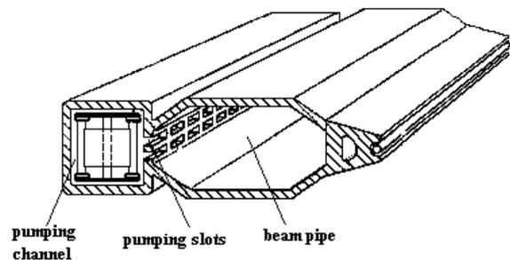
Fig. 1: A sketch of the dipole vacuum chamber in PETRA [3]
