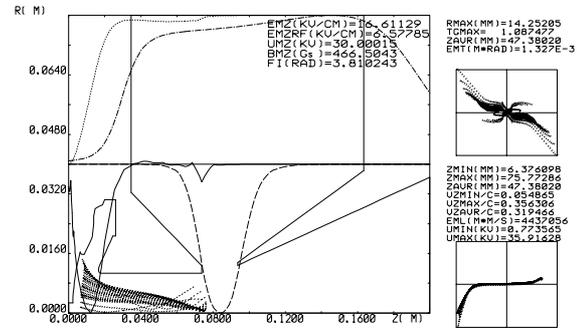
Figure: 3 SMASON calculation: bunch in front of cavity.
