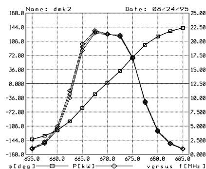
Figure: 6 Calculation of passband by KOP.
