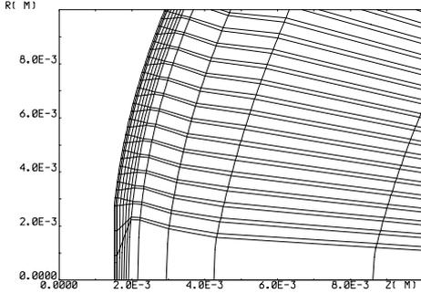
Figure: 1 Finite element mesh near cathode-grid region.
