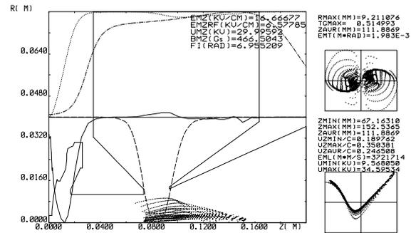
Figure: 4 SMASON calculation: bunch in the cavity gap.
