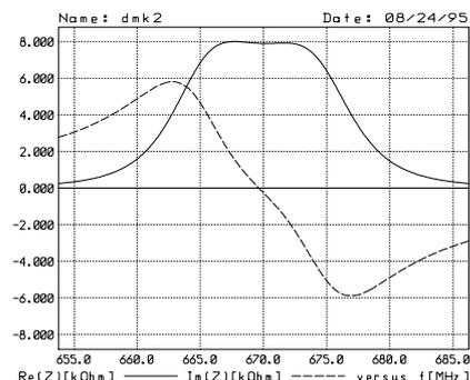
Figure: 5 Impedance of coupled cavities calculated by KOP.
