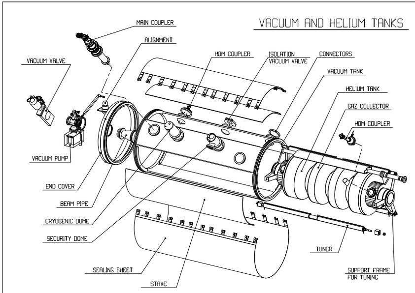
Fig. 1. Vacuum and helium tanks
