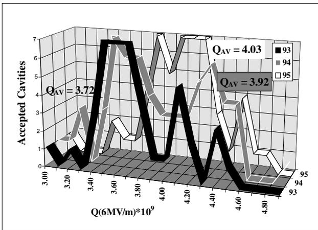
Fig. 5. LEP cavity performance vs. year of production
