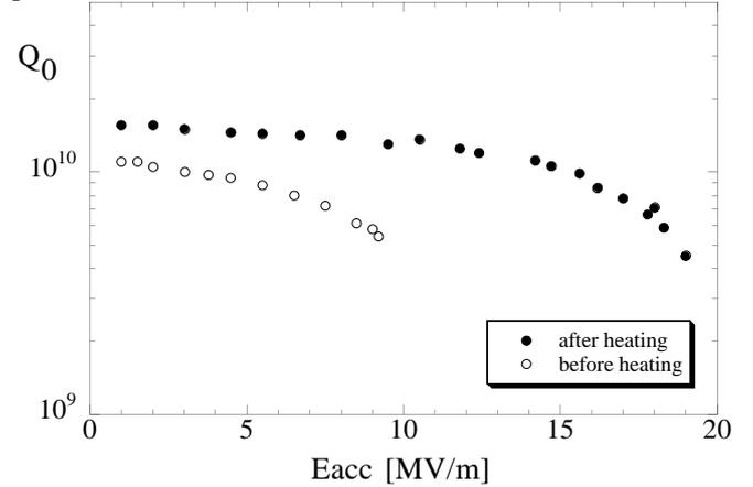
Fig. 3: Improvement of a single cell cavity after heat treatment with Ti at 1400 °C for 4 h (Saclay [13]). Several single cell cavities were limited by a quench at the equatorial weld. After heat treatment all cavities showed improved performance. There is evidence, that due to imperfect weld preparation enhanced contamination was collected at the weld and initiated excessive heating. During heat treatment the contamination was probably diluted and thus the bulk Nb was homogenised.
