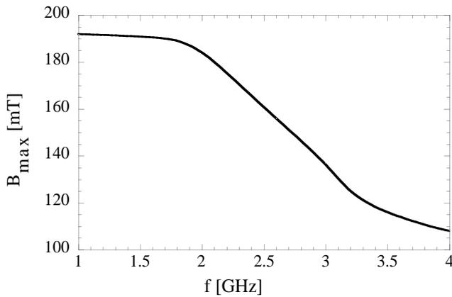
Fig. 1: Model calculation of thermal instability due to global heating by the surface magnetic field as function of frequency (Nb wall thickness 1.5 mm,  $\lambda_{4.2K}$  of Nb is 60 W/mK,  $T = 1.8$  K) [11]. The strong frequency dependency is expected because of the quadratic frequency term in the BCS surface resistance (see equ. 1).
