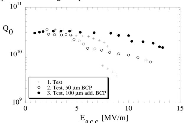
Fig. 6: Behaviour of a "bad" cavity (9-cell, TTF) with two additional surface treatments by BCP (buffered chemical polish). The signature is a jump in  $Q$  ( $Q$ -switch) and a decrease of  $Q$  when raising the field. This behaviour is most likely due to a defect in the bulk Nb because the cavity performance improved somewhat after surface removal (50  $\mu\text{m}$ , 100  $\mu\text{m}$ )
