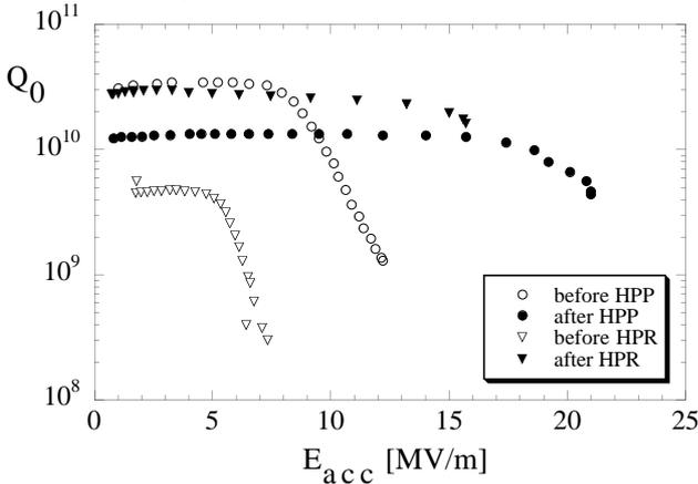
Fig. 2: Benefit of HPP (high RF power processing) and HPR (high pressure water rinse). Two different TTF cavities have been measured before (open points) and after (closed points) treatment by HPP and HPR, respectively.
