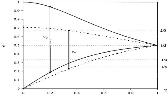
Figure 2 : Resonances excited by a mismatch versus  $\eta$ . Each pair of curves defines the range of resonances ( $v = 2/3...$ ) excited by the even ( $v_e$ ) and odd ( $v_o$ ) modes.
