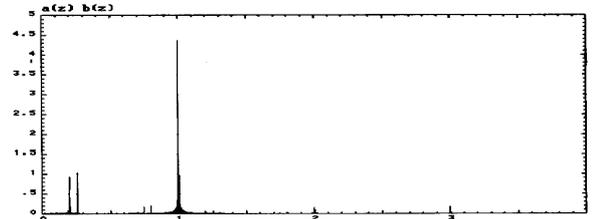
Figure 1 : Fourier spectrum of a mismatched beam envelope in a FODO channel. The intrinsic quadrupolar mode frequency is  $f = 1$ , the two peaks at low frequency are the two eigen modes.
