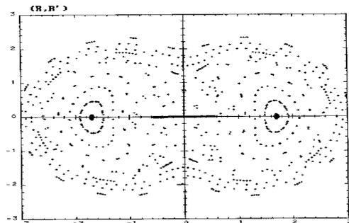
Figure 4 : Poincaré surface of section for  $\eta = 0$  [11]. The two  $v_e = 1/2$  islands are surrounded by "KAM tori" which limit the chaotic area.
