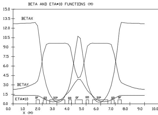
Fig. 2. MAX II machine functions.
