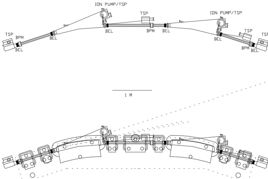
Fig. 1. One magnet cell.
