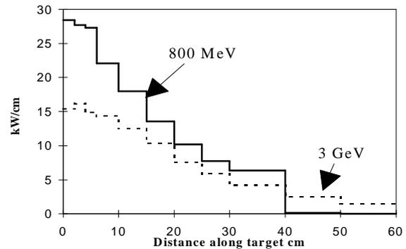
Figure 2. The power deposited along a lead target.
