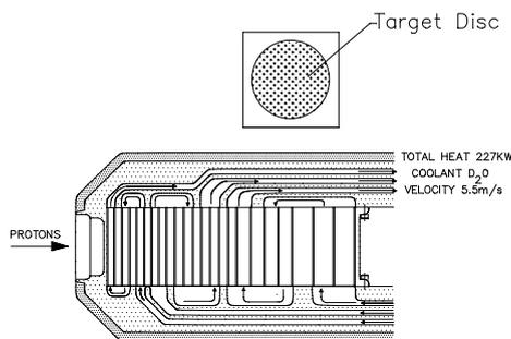
Figure 5. A schematic view of the ISIS target.
