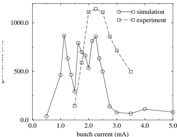
Fig. 2. Calculated and observed growth rate vs. bunch current for the lowest frequency mode.
