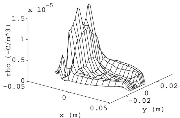
Fig. 1. Calculated trapped electron charge density, shown 10 ns after a bunch passage.
