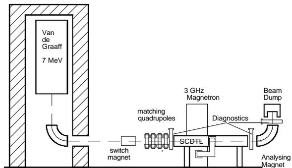
**Figure 7.** Layout of the experiment of protons acceleration by SCDTL at LNL
