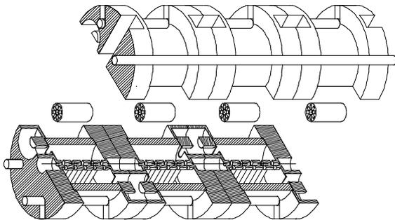
Figure 1 Longitudinal section of three tanks of the SCDTL
