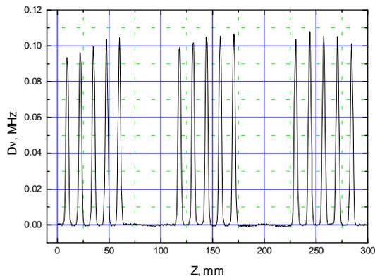
**Figure 5** Results of an axial bead-perturbation measurement for the  $\pi/2$  mode of the 5-cell SCDTL model
