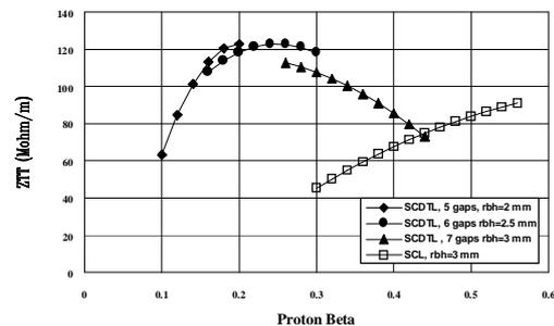
Figure 2 Computed values of the effective shunt impedance of a multigap DTL cavity operating in zero-mode and SCL cavity operating in  $\pi/2$  mode versus the particle  $\beta$ .
