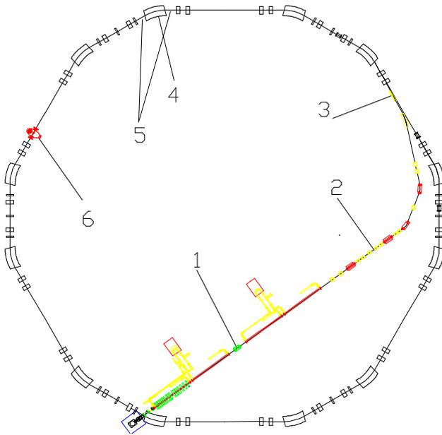
Fig. 4 Top view of the ring with linear accelerator, underground (1), transport line (2), thin septum (3), dipole magnet (4), PS (5) and RF cavity (6).
