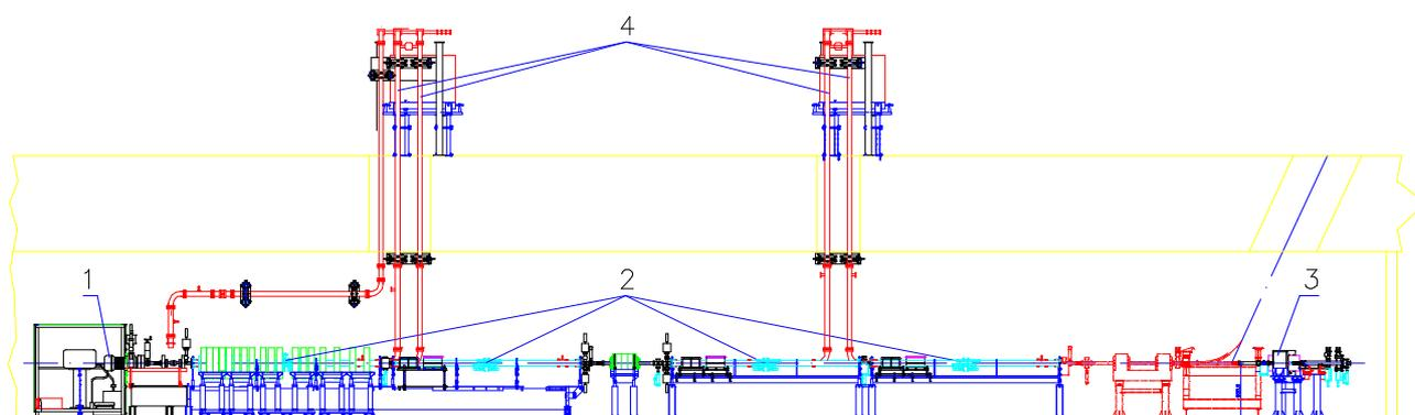
Fig. 1. Linac: CAD drawing of the gun (1), the linear accelerator structures (2), the spectrometer (3) and the wave guide of RF system (4)
