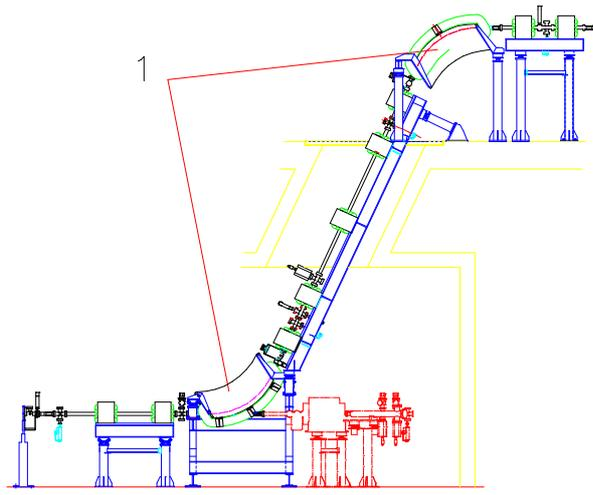
Fig. 2 Transition of under ground level and ring level, with 65° dipole (1) for deflection
