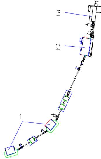
Fig. 3 Top view of transport line in the ring level with 33° dipole (1), the thick septum (2) and thin septum (3)
