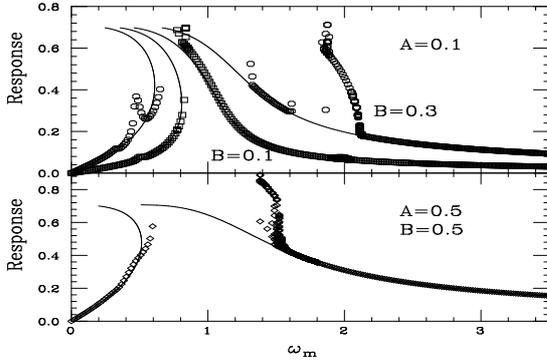
Figure 2: The amplitude of the steady state solution, called response, obtained numerically is plotted as a function of  $\omega_m$  for  $A = 0.1$  (upper plot), with modulation amplitudes  $B = 0.1$  (rectangles),  $B = 0.3$  (circles) respectively, and for  $A = 0.5$  (lower plot) with  $B = 0.5$ .
