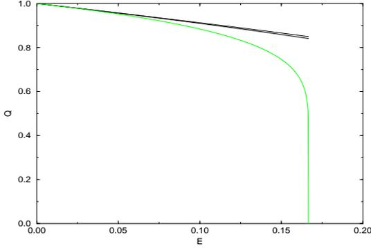
Figure 1:  $Q(E)$  vs  $E$ . The first order and the second order detuning terms are also shown. Because of the sharp drop of the synchrotron tune  $Q(E)$  around the separatrix, parametric resonances of all orders overlap with each other near the separatrix trajectory and give rise to stochasticity.
