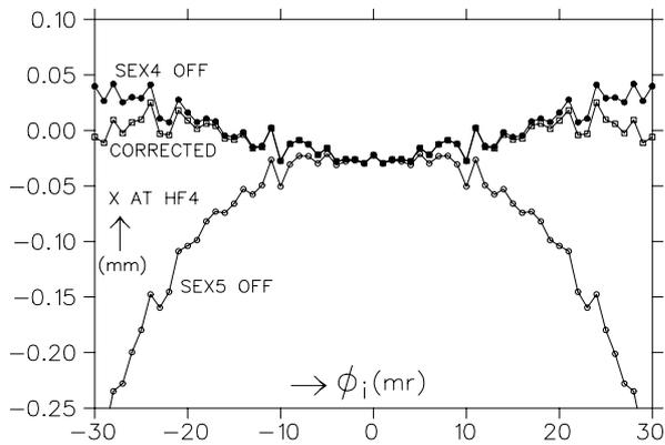
Figure 4: The influence of sextupoles SEX4 and SEX5 on the horizontal displacement in the final focal plane as function of the launching angle  $\phi_i$  at the source. SEX4 has almost no influence on  $\phi$ -related aberrations.
