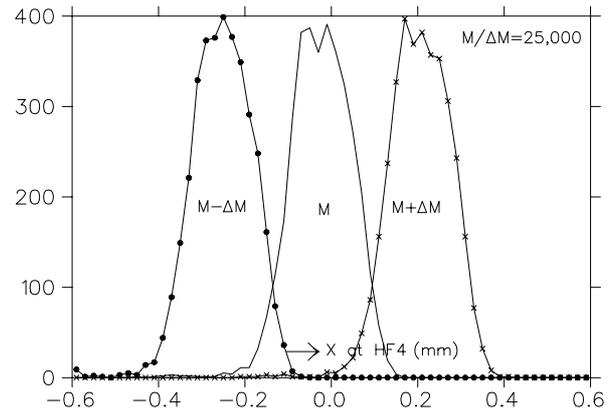
Figure 5: Mass resolution from higher order calculations.
