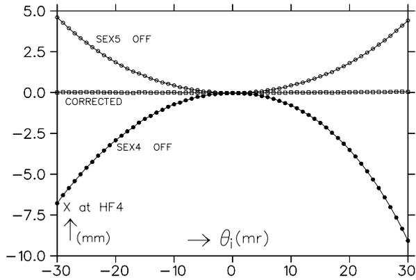
Figure 3: The influence of sextupoles SEX4 and SEX5 on the horizontal displacement in the final focal plane as function of the launching angle  $\theta_i$  at the source.
