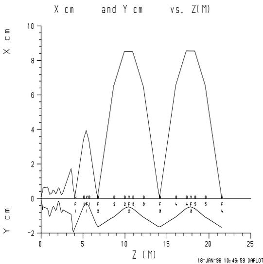
Figure 2: Beam envelopes in separator
