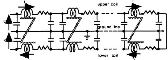
Figure 1: An equivalent circuit of the HIMAC magnet string.
