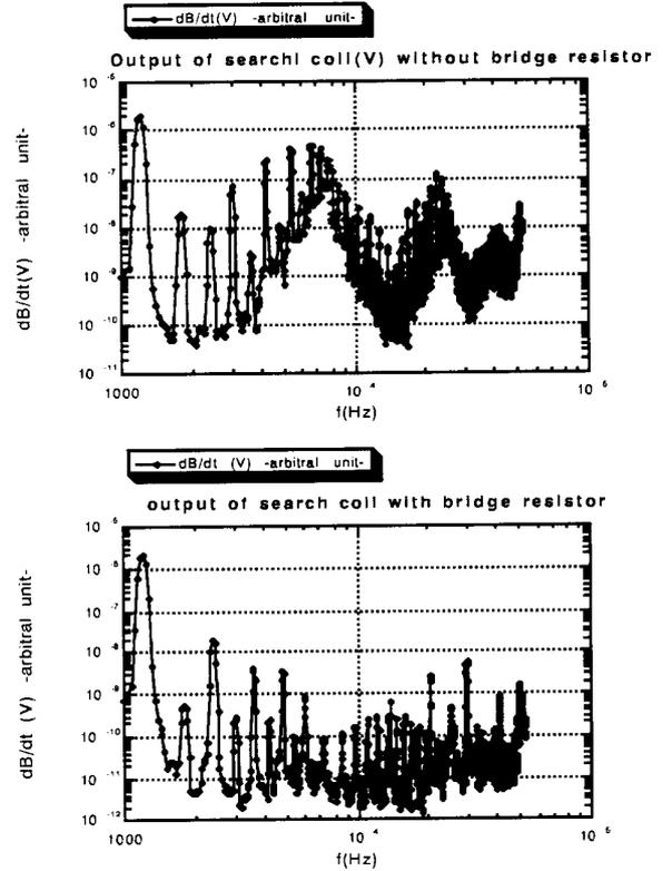
Figure 4: Ripple in search coil with and without bridge
