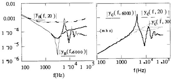
Figure 2: Admittance of the normal and the common mode with various magnitude of bridge resistor.
