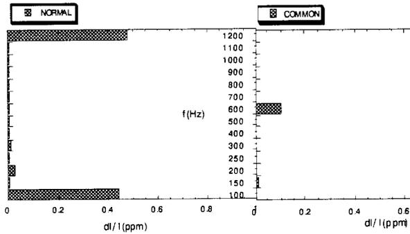
Figure 5: Current ripple measured in the bridge resistor
