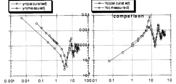
Figure 3: Admittance from the measurement and the calculation of normal and the common mode
