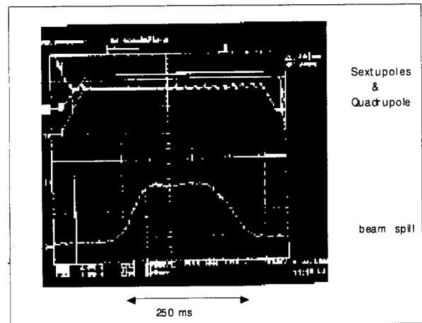
Figure 6: Figure 6 An example uniform beam spill
