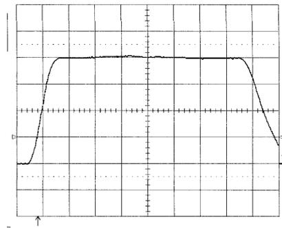
Figure: 7 Magnetic field in the core gap of a short-ended kicker magnet. (X:200ns/div, Y:8.8\*10<sup>-3</sup>T/div)
