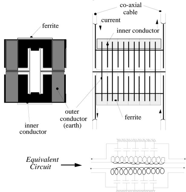
Figure: 4 Structure of the distributed twin kicker magnet.
