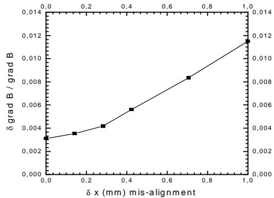
Figure 3 Influence of pole constructional asymmetry on the gradient
