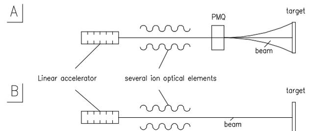
Figure 1 Schematic set-up of the irradiation facility
