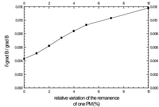
Figure 4 Influence of a relative decrease of the remanence of 1 PM (15 PMs keeping their remanence) on the gradient
