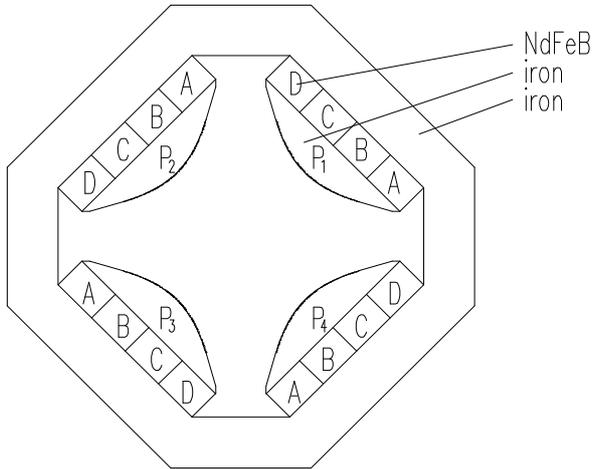
Figure 2 Sketch of the quadrupole
