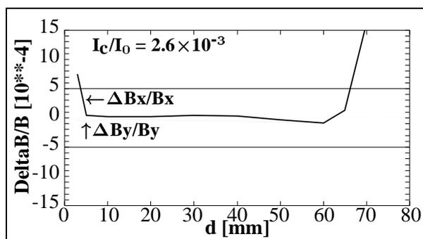
Figure 8:  $\frac{\Delta B}{B} = \frac{B - B_I}{B_I}$ , in units of  $10^{-4}$ , as function of distance from origin.  $B_I$  is field calculated for an ideal quadrupole given by  $B_I(d) = \text{Gradient} \times d$ .
