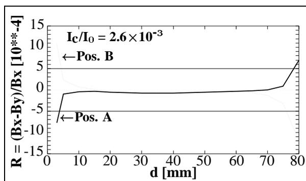
Figure 7: Field difference ratio  $R$ , in units of  $10^{-4}$ , as a function of distance  $d$  from origin. A and B refer to positions shown in Fig. 5.
