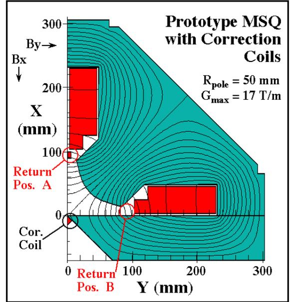
Figure 5: MSQ with 45° cut in 70 mm thick mirror plate mounted on half QC-type quadrupole. Correction coil is placed near center with possible return positions as indicated at points A and B.
