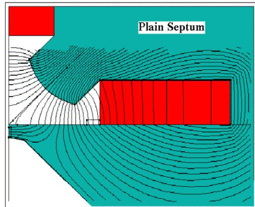
Figure 1: Center of MSQ with 45° cut ending at 10 mm septum thickness. Only right half shown due to horizontal symmetry.
