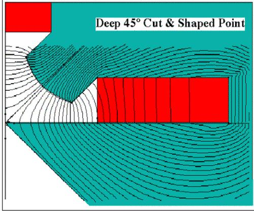
Figure 3: MSQ with 45° cut extending to origin.
