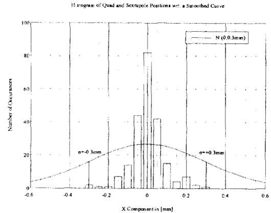
Fig.6 Histogram of the lateral displacements of quadrupoles and sextupoles of the booster synchrotron
