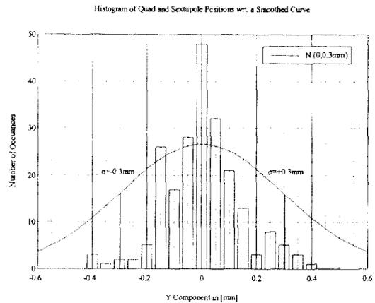
Fig. 7 Histogram of the vertical displacements of quadrupoles and sextupoles of the booster synchrotron
