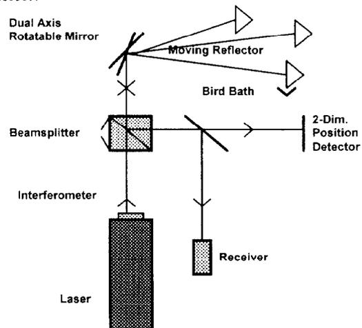
Fig. 2 Optical path of the SMART 310 Laser Tracking System
