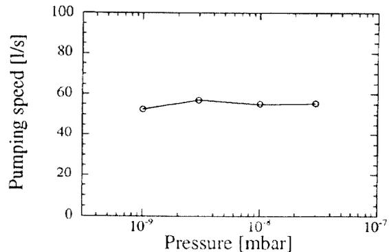
Figure 5. Pumping speed of the prototype of the distributed sputter ion pump working at 1 T.
