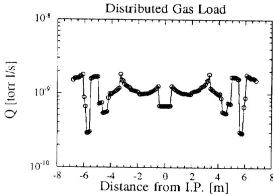
Figure 3. Gas load distribution along the vacuum chamber.
