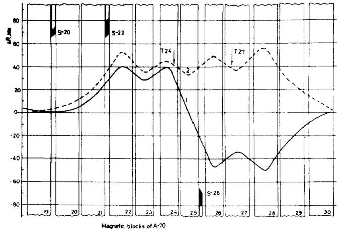
Figure 1: The form of the closed orbit local distortions under simultaneous operation of targets.
