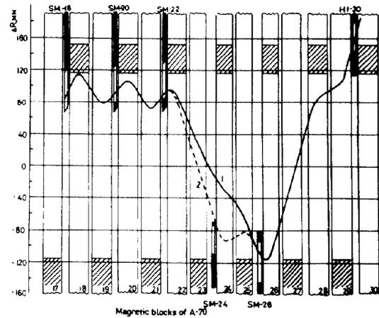
Figure 3: The trajectories of a proton beam being extracted in NRSE regime (a current of the SM-22 is a calculated one) simultaneously to internal targets operation. 1—T27 on negative coordinates; 2—on positive ones.
