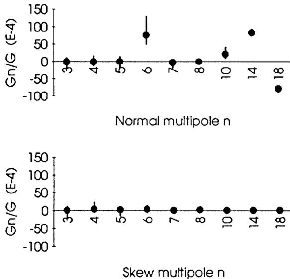
Fig.3. Integrated multipoles measured at radius 59 mm
