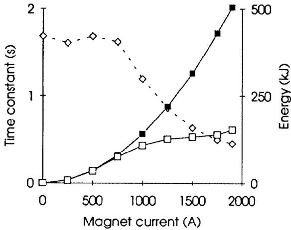
Fig. 2. Quench back when unloading over dump resistor
