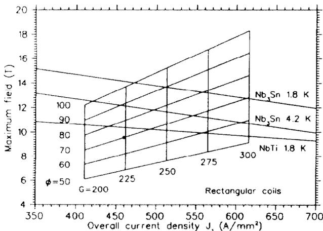
Figure 3: Quadrupole gradient  $G$  (T/m) and aperture  $\phi$  (mm) as a function of current density and peak field in the inner blocks. Critical current curves for  $Nb_3Sn$  and  $NbTi$  cables are also shown. The dot indicates the reference design.
