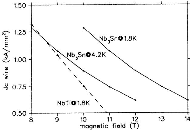
Figure 1: Critical current density vs field for NbTi/Cu and Nb<sub>3</sub>Sn/Cu wires. The Cu:non Cu is 1.35 for NbTi and 1.0 for Nb<sub>3</sub>Sn . A 3 % cabling degradation for NbTi and 10 % for Nb<sub>3</sub>Sn has been taken into account.
