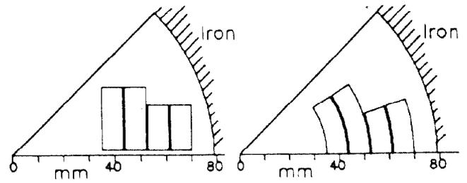
Figure 2: Schematic view of a four blocks quadrupole with rectangular or shell coil geometry. See text for details.
