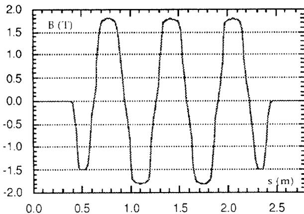
Figure 3. Vertical field along the wiggler axis
