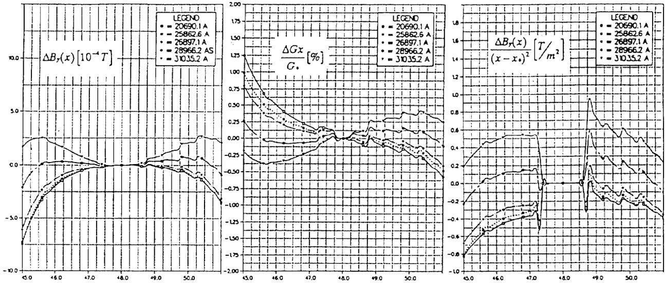
Fig. 2. Flux density and gradient deviations as well as sextupole component for the ROSY dipoles
