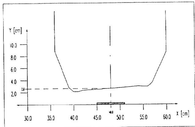
Fig. 1. Pole face of the optimized ROSY dipol
