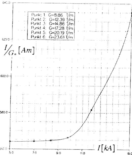
Fig. 5. Ratio of excitation current to orbit gradient for the ROSY quadrupoles as function of the excitation current
