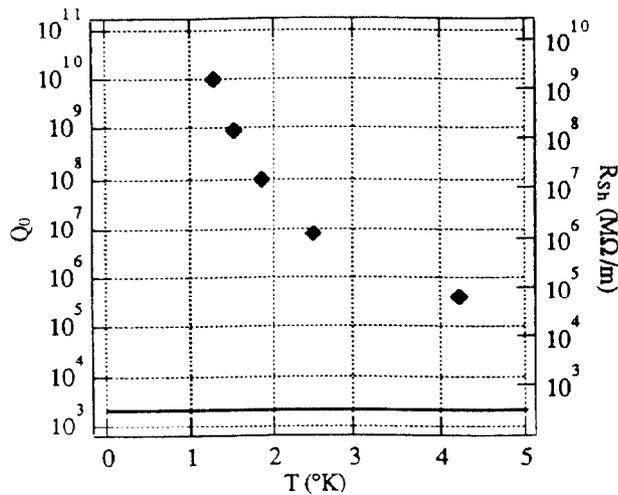
Figure 2 Unloaded quality factor  $Q_0$  and shunt impedance  $R_{sh}$  of the accelerating structure, at various temperatures for superconducting niobium.
