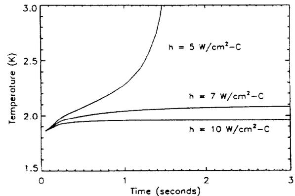
Figure 3. Typical increases of the maximum temperature, as a function of time for various effective film coefficients.
