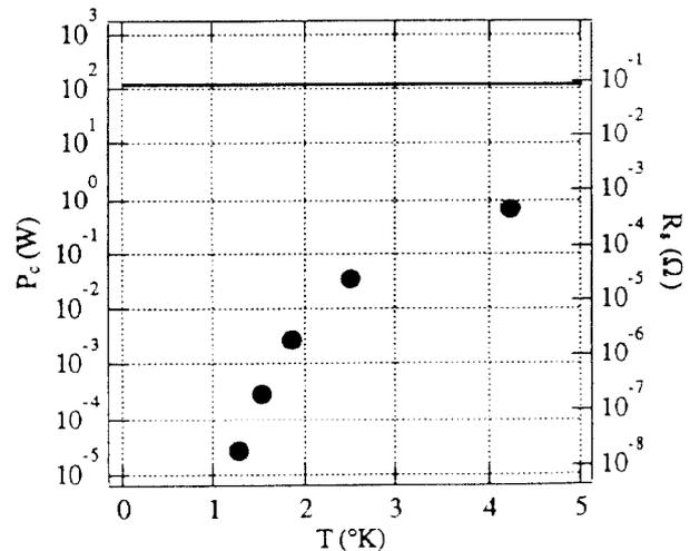
Figure 1. Surface resistance  $R_s$  of the cavity walls and the corresponding power losses  $P_c$  of one cavity, at various temperatures of superconducting niobium.
