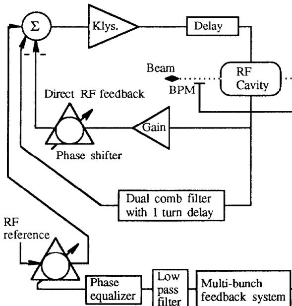
Figure 4. Block diagram of RF feedback circuits
