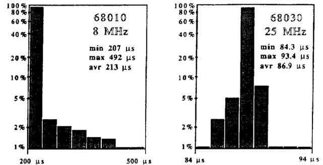
Figure 3. Measured statistical distribution of the delay time between the broadcast generation and the DAC setting.
