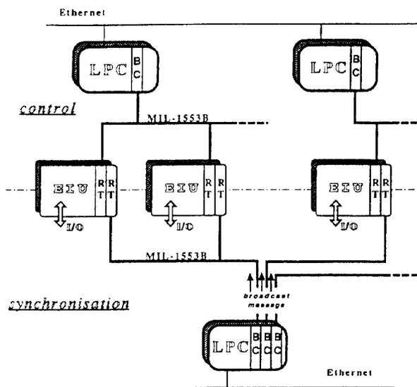
Figure 2. The control and synchronisation systems.
