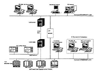
Figure 1: The general control system layout
