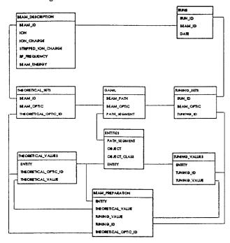
Figure 3: Overview of the beam parameter database
