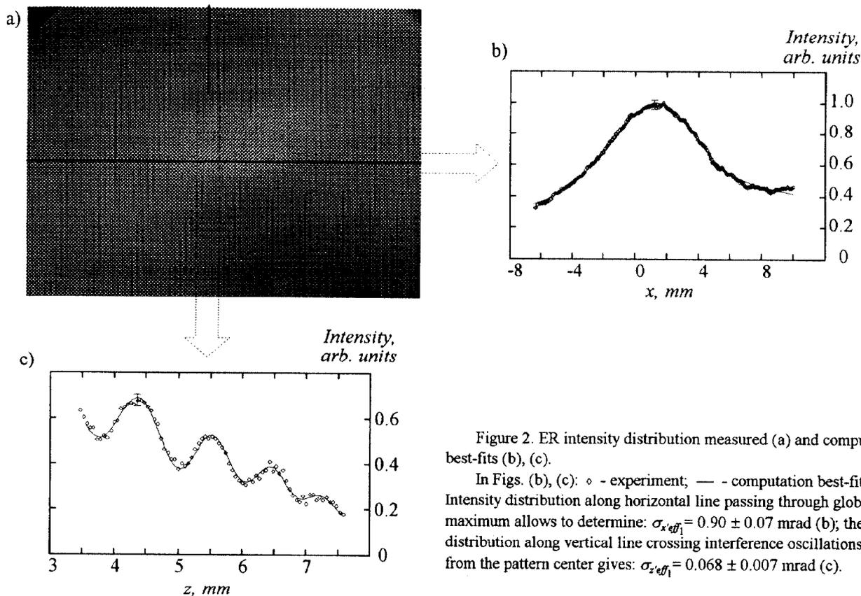
Figure 2. ER intensity distribution measured (a) and computed best-fits (b), (c).
