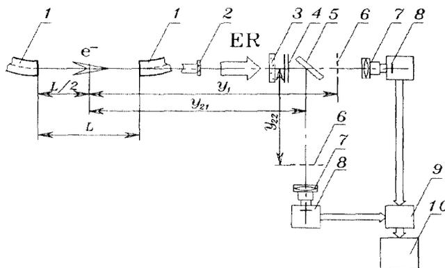
Figure 1. Scheme of the ER measurement system.
