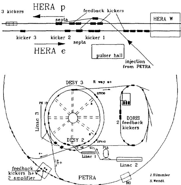
Figure 1. Feedback kickers in the machines
