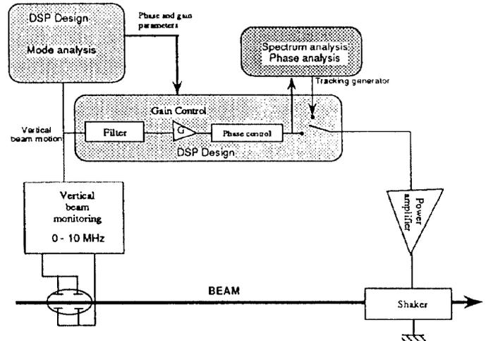
Figure 2: Single Bunch feedback layout
