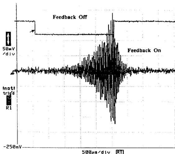
Figure 4:  $\Delta Z$  Motion, Feedback On/Off
