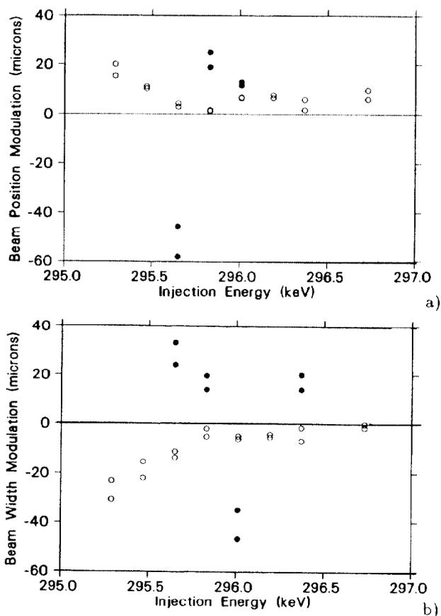
Fig. 2(a). Beam position peak-to-peak modulation at 223 MeV, versus energy at injection to the cyclotron. The beam lines and cyclotron were initially optimized for approximately 296 keV injection energy. Solid circles, bunchers on,  $\pm 6$  V applied modulation. Open circles, bunchers off,  $\pm 30$  V applied modulation. (b) Beam width peak-to-peak modulation, same conditions as 2(a).
