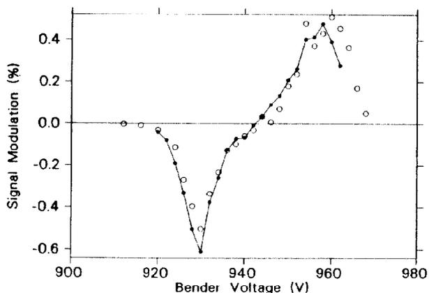
Fig. 1. Instrumental signal response to applied  $\pm 30$  mV voltage modulation (solid line) compared with helicity-correlated signal modulation at 2.8 keV.
