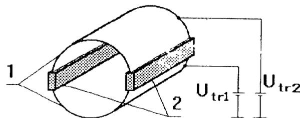
Fig. 1 - The schematics of the electrostatic trap.
