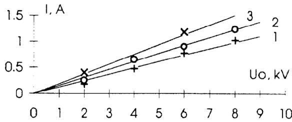
Fig. 2 - The dependence of the upper current limit on the accelerating voltage. 1)  $P = 3 \times 10^{-9}$  Torr, 2)  $P = 6 + 8 \times 10^{-8}$  Torr, 3)  $P = 1.5 + 4 \times 10^{-7}$  Torr.
